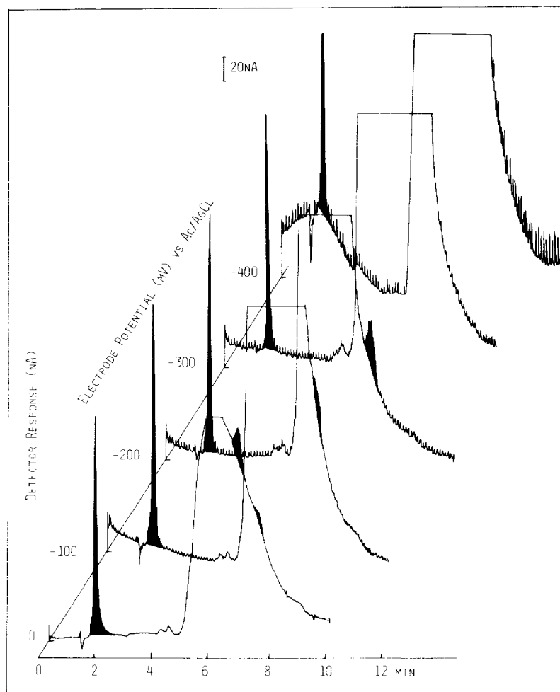
Fig. 6. Variation of cell current as a function of applied potential ( E ). The resultant effect on the chromatogram of 25 \mu\text{l} aged CDDP (5.5 \mu\text{g/ml} ) for the potential range 0.0 mV to -400 mV vs. Ag/AgCl.
